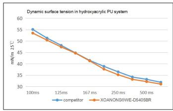
Dynamic surface tension (DST) is measured by bubble tensiometer. This parameter is representative in coating application (such as spraying). It measures the surface activity of coating additives in the coating process, that is, the diffusion ability of coating additives from solution to interface. The smaller the dynamic surface tension, the faster the leveling speed of the coating under the same time conditions.
