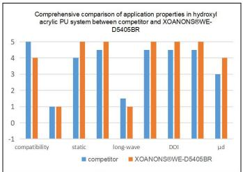
Dynamic friction coefficient for slip (  $\mu$  d). The lower the value, the 5 = excellent 0 = poor better the slip and feel. Excellent slip will bring good scratch resistance and improve anti adhesion.
