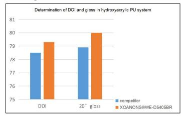
The freshness and gloss are measured by orange peel tester and triangle gloss tester respectively.
