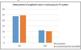
The long and short waves are measured by orange peel instrument. LW is long wave comprehensive data. The lower the value, the better the long wave level; SW is short wave comprehensive data. The lower the value, the better the short wave level.
