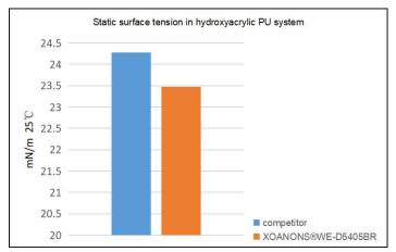
The static surface tension is measured by automatic surface tension meter. This parameter measures the ability of coating additives to wet and spread on solid surfaces under balanced surface tension. The smaller the static surface tension, the stronger the wetting and spreading ability.
